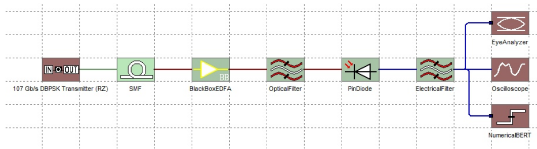
Figure 3.9.2. A typical setup to carry out BER estimations for a DBPSK system (one span).
